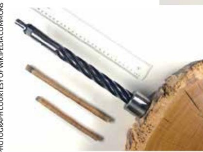
A dendrochronological drill bit designed to make core samples for accurate laboratory analysis. Frequently used to date timbers in ancient wooden structures such as timbered houses, barns and ships
