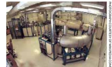
An accelerator mass spectrometer at Lawrence Livermore National Laboratory used for carbon dating. Dendrochronological samples can be used as reference markers to help improve the accuracy of carbon dating
